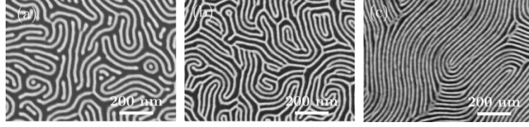
Figure 7.28. SIS with \text{Al}_2\text{O}_3 on PS- b -PMMA as a function of BCP chain length: (a) 38 nm, (b) 28 nm, and (c) 22 nm (SEM images have been taken after PS removal)
